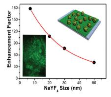
An "islands" Au-Ag/NaYF4: Yb3+, Tm3+ composite film is prepared by an organic self-assembly and removal template method. The Au-Ag alloy has the stable and repeatable properties and exhibits super-broad surface plasmon resonance band extending to 1100. It obtained ≈180fold enhancement of upconversion luminescence for fingerprint identification.
