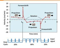
The direction of self-propulsion of diodes floating on a water surface, powered by external alternating (AC) electric fields, can be controlled on-demand by electronically modifying the symmetry of the applied AC waveform. Changes in the duty cycle of the signal inducing short-lasting DC fields can be used to remotely reverse its direction of motion or make it move sideways.
