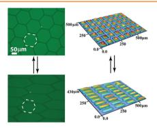
Chemically patterned silicone films drive the assembly of microdroplets into ordered arrays. These microdroplets can be "stretched", a capability that was used to drive mixing in the droplets and to change the lensing characteristics of the array. Synthesizing "stretchable" chemical patterns of different geometries and functional groups provides a method to explore soft, mechanoresponsive surfaces with rapidly reversible properties unavailable in hard systems.
